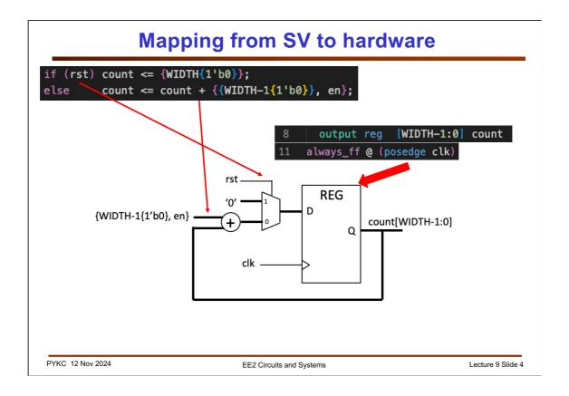
This is how the SV code is mapped to the actual hardware synthesized by Verilator.
