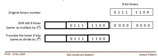
Before we examine this algorithm in detail, let us consider the arithmetic operation of shifting left by one bit. This is the same as a  $\times$  2 operation. If we do it 8 times, then we have multiplied the original number by 256 or  $2^8$ .
