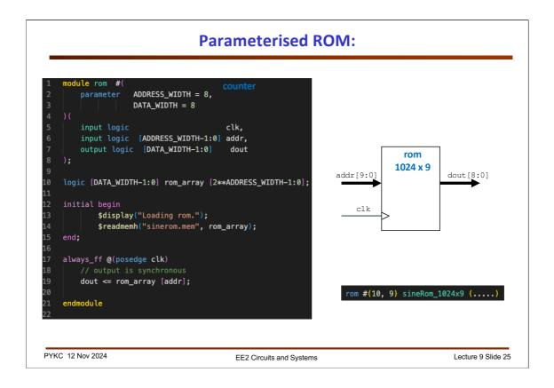
Note that **rom.sv** is defined with two parameters: **ADDRESS\_WIDTH** and **DATA\_WIDTH**. These are given default values. However, if you need a ROM that is 1024 x 9 bit instead of 256 x 8 bit, you can simple specifiy these parameter as shown here when instantiating the ROM component. The order of the parameters is important!
