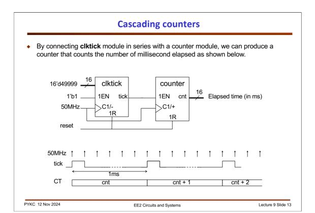
Using this style to design a clock tick circuit allows us to easily connect multiple counters in series as shown here.
