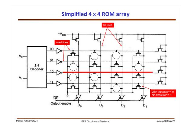
This is a simplified internal circuit of a 4 words x 4 bits Read-Only Memory (ROM) component.
