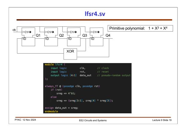
Here is the implementation of a 4-bit LFSR of the primitive polynomial
