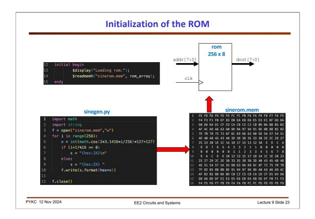
ROM needs to "programmed" or configured with original contents. In SystemVerilog, the **\$readmemh(.)** function allows the ROM to be loaded with the contents stored in a file with numbers stored as hexadecimal code as shown in the slide.
