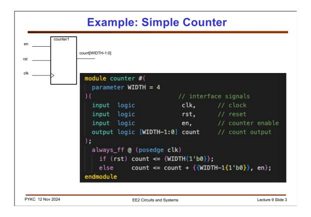
In Lab 4, you are to design an 4-bit counter as shown here. The counter has three inputs:
