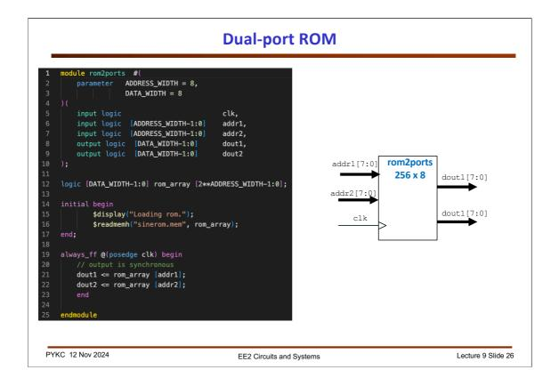
In designing on-chip memory for microprocessors, we often need to perform more than one access operations simultenously to the same memory. Here is a specification for a dual-port ROM. The actual SystemVerilog code is very simple and obvious. Now a user can read from two separate memory location at the same time.
