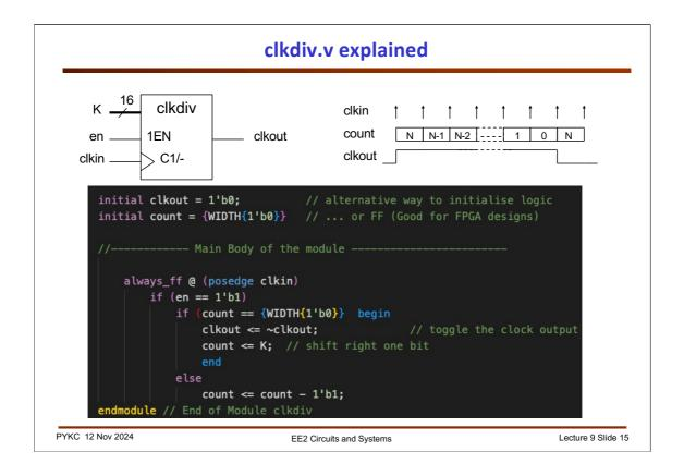
The Verilog specification is similar to that for **clktick**. This also has an internal counter that counts from K to 0, then the output **clkout** is toggled whenever the count value reaches 0.
