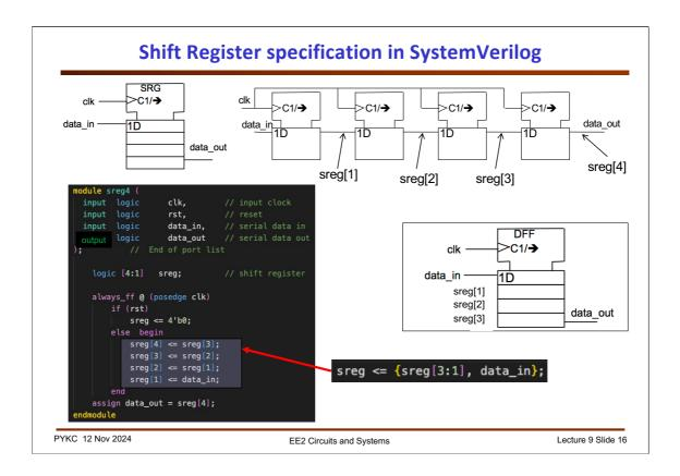
To specify a shift register in SystemVerilog, use the code shown here. We use the <= assignment to make sure that **sreg[4:1]** are updated only at the end of the **always** block.
