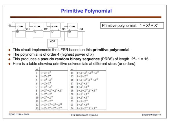
The circuit shown below is effective implementing a sequence defined by a polynomial shown:  $1 + X^3 + X^4$ . The term "1" specifies the input to the left-most D-FF. This signal is derived as an XOR function (which is the finite field '+') of two signals "tapped" from stage 3 (i.e.  $X^3$ ) and stage 4 (i.e.  $X^4$ ) of the shift register.
