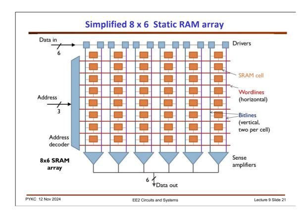
This slide shows a typical organisation inside a RAM chip. Memory cells are usually organised in the form of a 2-D array of RAM cells. In this case, the address is 3 bits, therefore there are 8 words in this memory. Only ONE ROW will be enable at any one time (hence one-hot).
