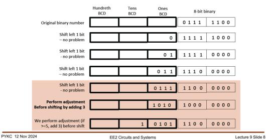
The rationale of this algorithm is the following. If the number is 5 or larger, after shift left, we will get 10 or larger, which cannot fit into a BCD digit. Therefore if the number 5 (or larger) we add 3 to it (after shifting is adding 6), which measure we carry forward a 1 to the next BCD digit.
